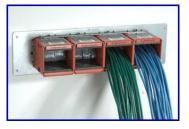
For example, the typical column pressure occurring in an enclosure with an FM200<sup>TM</sup> system would be around 10-15 Pa. At these pressures, an empty Series 22 device will add approximately .08 in<sup>2</sup> (0.50 cm<sup>2</sup>) leakage to the enclosure while a fully loaded Series 22 device will add approximately 0.09 in<sup>2</sup> (0.58 cm<sup>2</sup>).
